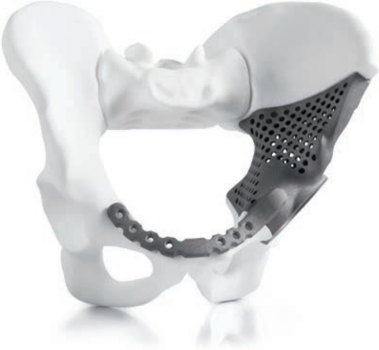
The titanium implant has a large number of cavities. These weight-reducing recesses in otherwise solid parts can only be achieved through Additive Manufacturing (courtesy of EOS GmbH).
