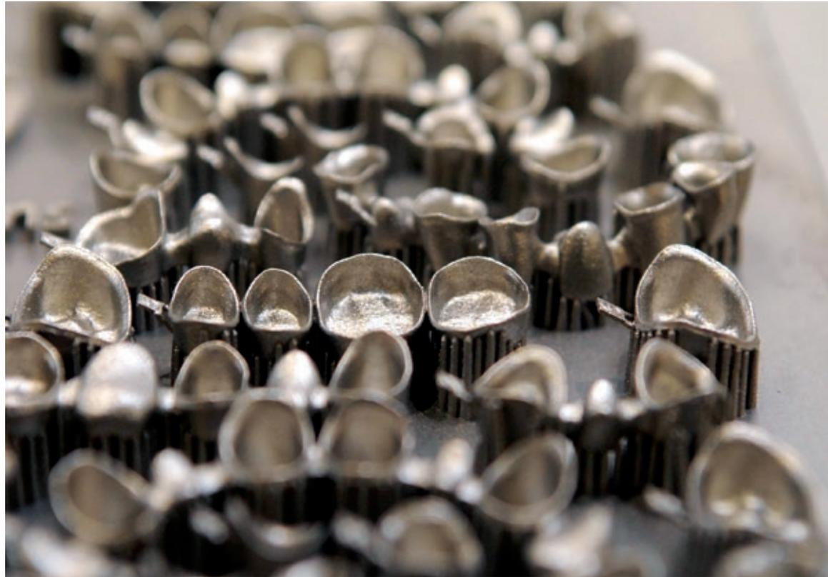
*Thin cross-sections of alloy powder are sequentially melted by a laser driven by this geometry, automatically building complete 3D restorations with structural fixtures not yet snapped off (Source: EOS GmbH).*
